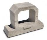
The 4 x 2" anchor bar on the underside of Premier 6 creates an automatic 0.5" (4.7°) setback with the highest shear resistance in the industry.
