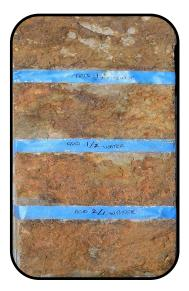
This sample shows an acid etch stain, with varying stain to water dilution ratios.
