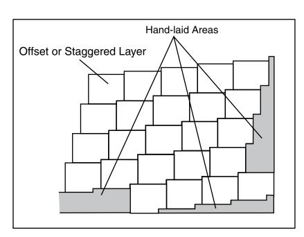
Figure 9. Staggered installation of clusters (8).
