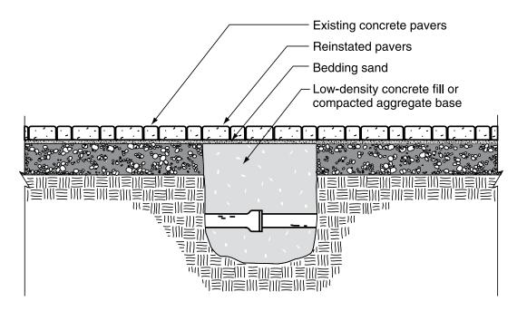
Figure 6. Cross section of reinstated utility cut into interlocking concrete pavement.
