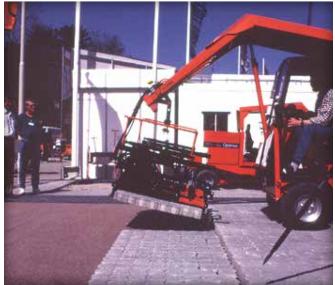
Figure 22. After the layers are separated they can be grabbed by the machine clamp.
