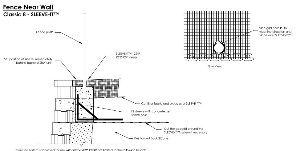
\*Fencing systems approved for use with SLEEVE-IT™ 1224R are limited to the following heights: Chain link - up to 8ft, Privacy: up to 6ft (Wooden, PVC, Metal). Post size 4"X4" max.
