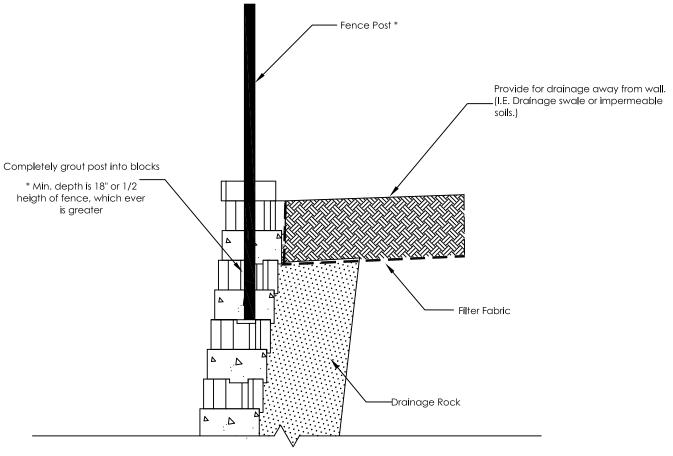
\*Non wind bearing fence. If lateral loads will be applied, fence should be designed by structural engineer.
