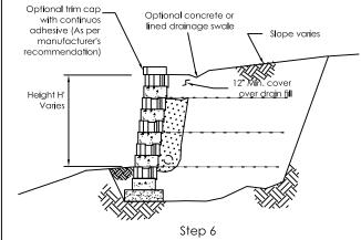
This drawing is furnished for preliminary design purposes only, and should not be used for final design drawings or construction drawings without the certification of a professional engineer registered in the state in which the wall will be constructed
