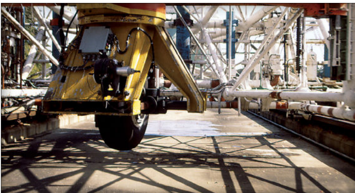
Figure 8. Test equipment for evaluation of the friction properties of concrete pavers at NASA's Aircraft Dynamics Landing Facility (ADLF) in Langley, Virginia
