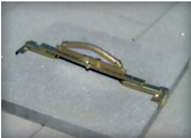
Figure 10. Single hand scissor clamp for lifting small and thin paving slabs
