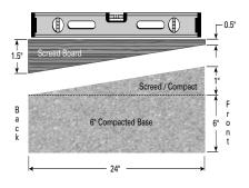
Simply place 1" of material on top of your compacted leveling pad. Screed the excess material away using
